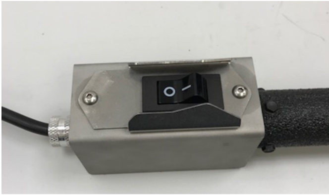
Rocker switch on handle end, in off position, acts as circuit breaker reset in case of over-current
