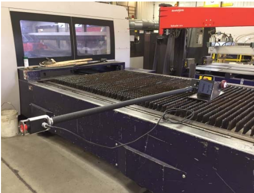
With switches off plug tool in
