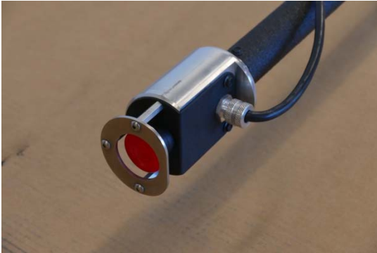
Red push button. Push in to turn off
