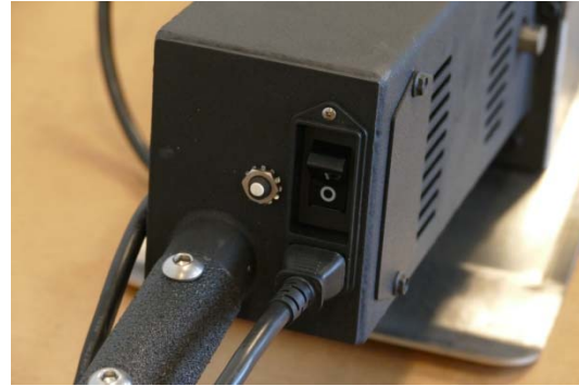
Rocker Switch on power unit in off position. Circuit breaker reset switch
